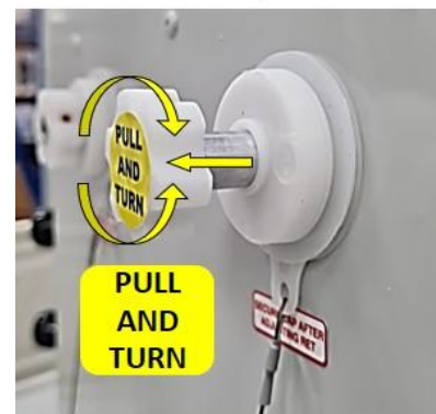
Pull handle out to disengaged RET for tilt adjustment
